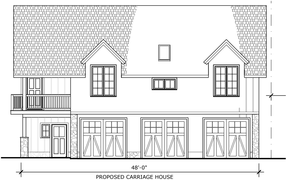
EXTERIOR ELEVATION - SOUTHEAST (FACING REAR OF (E) BUILDING)
